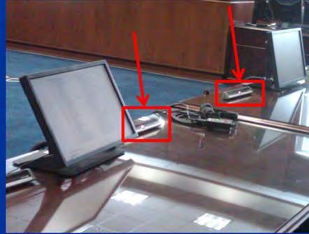
Let's take a look at the microphones first. Notice the **red** light. When they're red, they are set to ON **unless** you press the button, which is basically a "**push to mute**" button. So, if its not pressed, the microphone is active or **On**.
